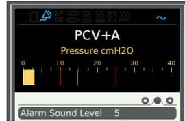
2 Press the Down or Up arrow button to select the Alarm Sound Level setting.
